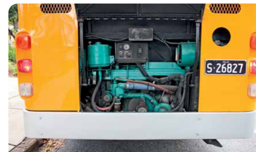
Top: A Volvo BR7LE/Volgren Optimus flashes past its ancestor out the front of the Toowong depot; Above: The 9.6-litre engine lays down and pushes out plenty of power and pollution
